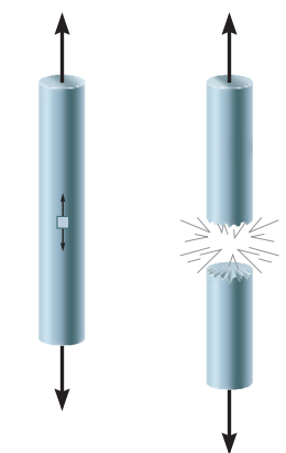
Failure of a brittle material in tension
